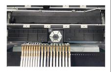
Upgraded to support 8-56mm NXT electric and vibration feeder
