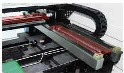
The XY Axis use Japanese servo motors,to control the repeated positioning accuracy error within 0.01mm,it also support mounting 0201 and pin pitch above 0.3mm QFP, BGA and etc.
