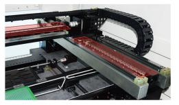
The XY Axis use Japanese servo motors, to control the repeated positioning accuracy error within 0.01mm, it also support mounting 0201 and pin pitch above 0.3mm QFP, BGA and etc.
